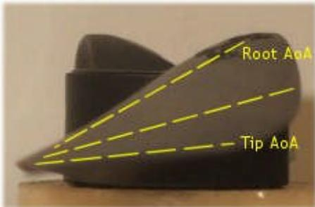
The 'twist' in the propeller is there to create the essential Angle of Attack of each blade, just like a wing has an AoA. The twist is greater towards the hub of the prop because of varying airspeeds along the length of the blades, and hence varying thrust generation.
