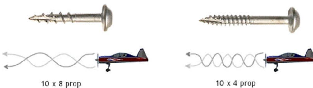
So you can see that selecting a different propeller pitch size is going to significantly change your airplane's performance, with speed being the primary factor.
