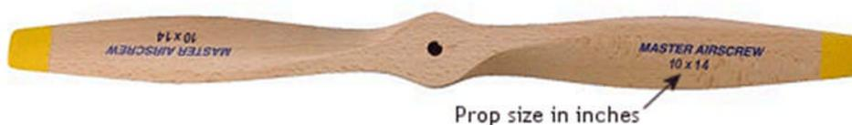
The first number is the **diameter** of the imaginary disc ('arc') created by the spinning prop *i.e.* the length of prop from tip to tip. The second number is the **pitch** and this is the harder of the two to understand – but we'll give it a go...
